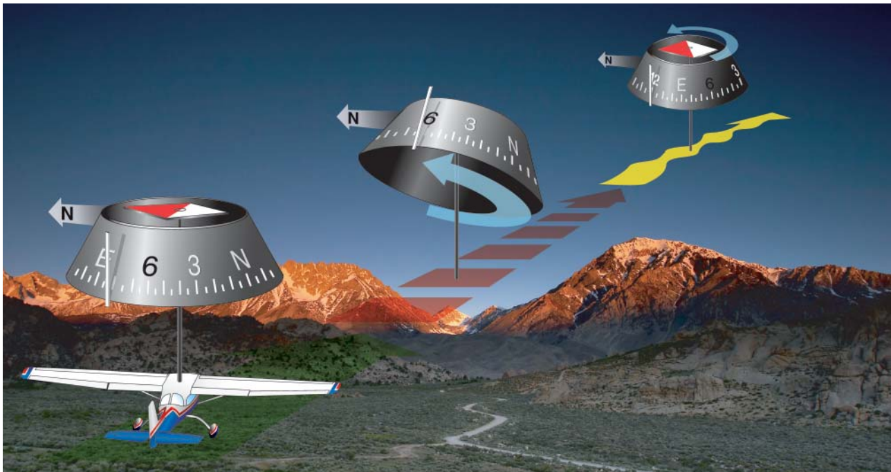
Figure 3-21. The Effects of Acceleration Error.
